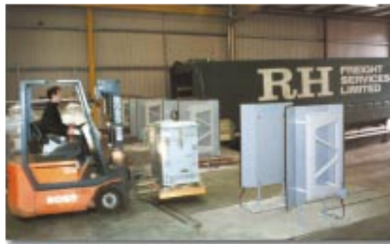
RFID tagged Xerox copiers pass through gate antennas to ensure they are loaded on the correct truck.
